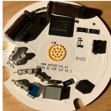
LED Module with IoT (DimIn Casambi)
