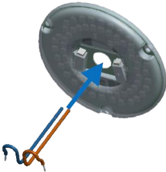
1 Insert the AC wire into the cover hole.
