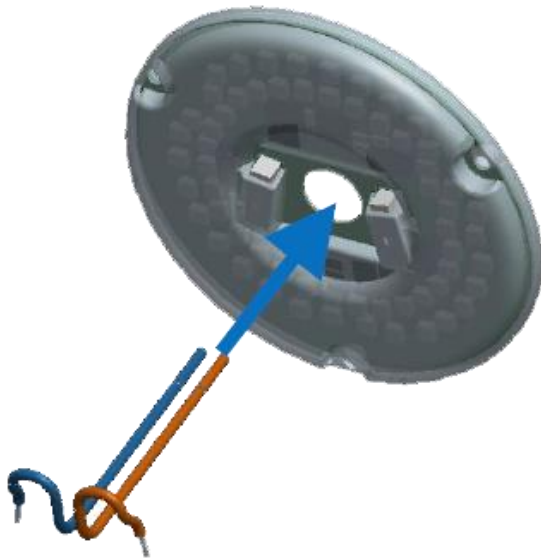
1 Insert the wires into the cover hole.
